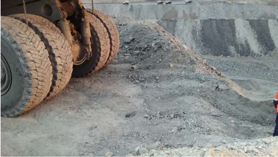
Photograph 3: The drill rig has trammed over windrow, showing the rig's position after it was pulled back from the edge. Photo courtesy of the mine.
