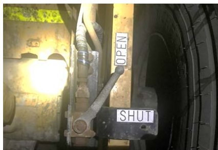
Figure 4. Hydraulic isolation valve handle in the open position. (Photograph by Resources Regulator)
