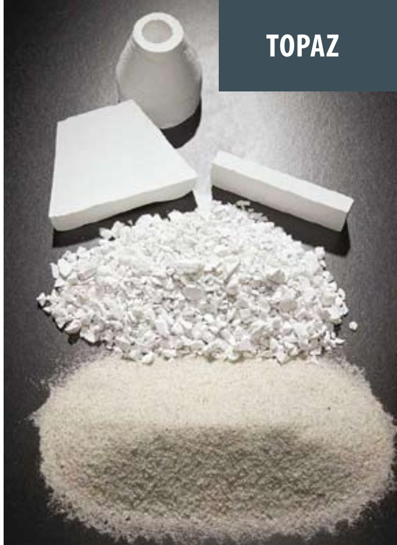
*Photograph 23. Topaz, mullite sand and products. The topaz was obtained from the Torrington silexite deposit, New England region. Mullite is a synthetic, fused (calcined) crystalline aluminium silicate produced in electric arc furnaces from alumina and silica for such applications as refractory tubes, industrial crucibles, analytical equipment and refractory cements. (Photographer D. Barnes)*
