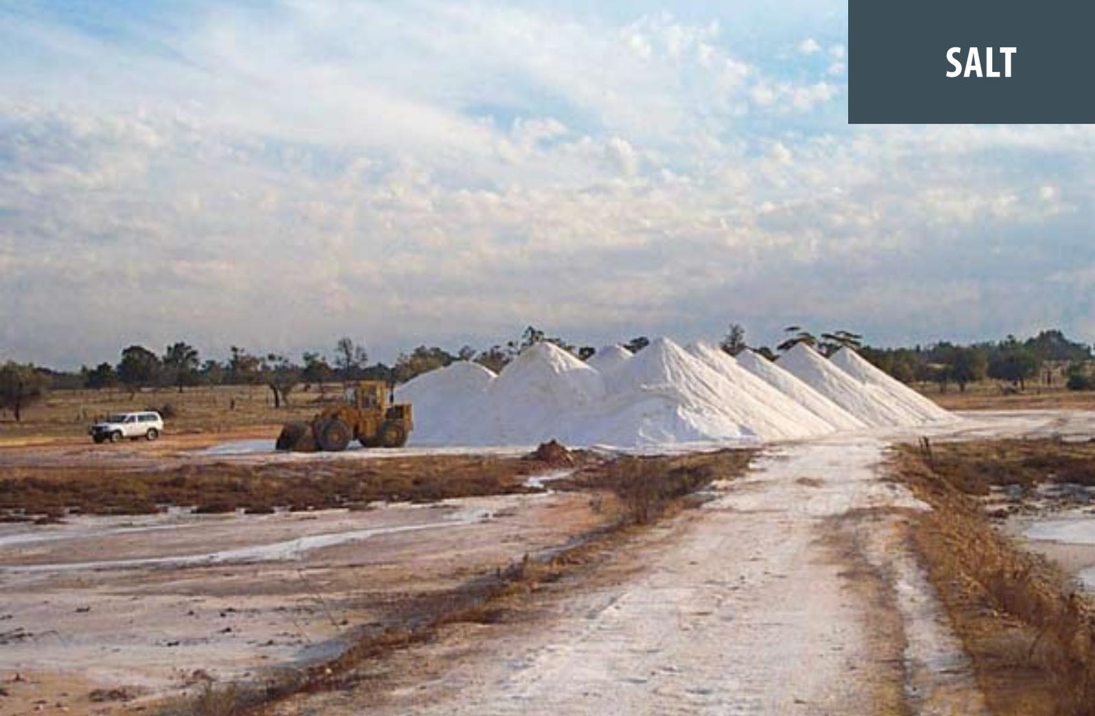
*Photograph 18. Raw salt stockpile, Mourquong Basin salt remediation scheme, northeast of Mildura. This salt was obtained by solar evaporation of highly saline groundwater pumped from shallow aquifers in the Murray Basin during salt remediation work. (Photographer J. Whitehouse.)*
