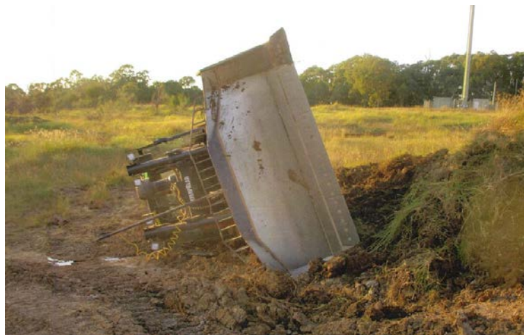
Figure 1: Cat D8 dozer after rolling off the bund (IncNot0033917). Photo courtesy of the mine.
