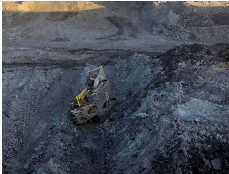
Figure 4: Dozer rolled into a slot (SInNot-2018/01730). Photo courtesy of the mine.
