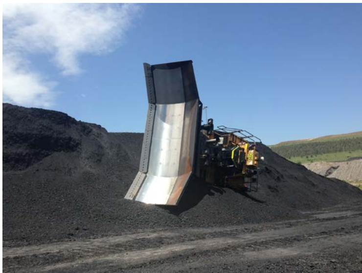
Figure 3: Dozer rolled on a coal stockpile (IncNot0033387). Photo courtesy of the mine.
