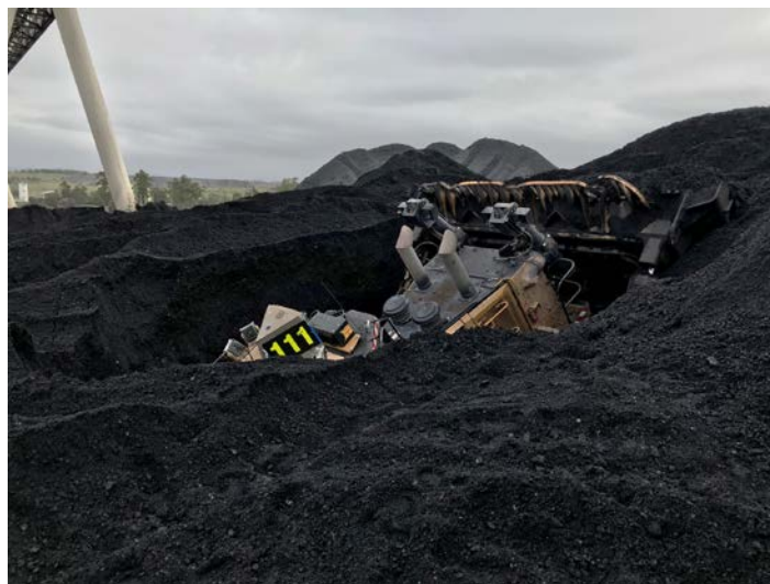
Figure 2: Dozer sunk into a void (IncNot0033728). Photo courtesy of the mine.
