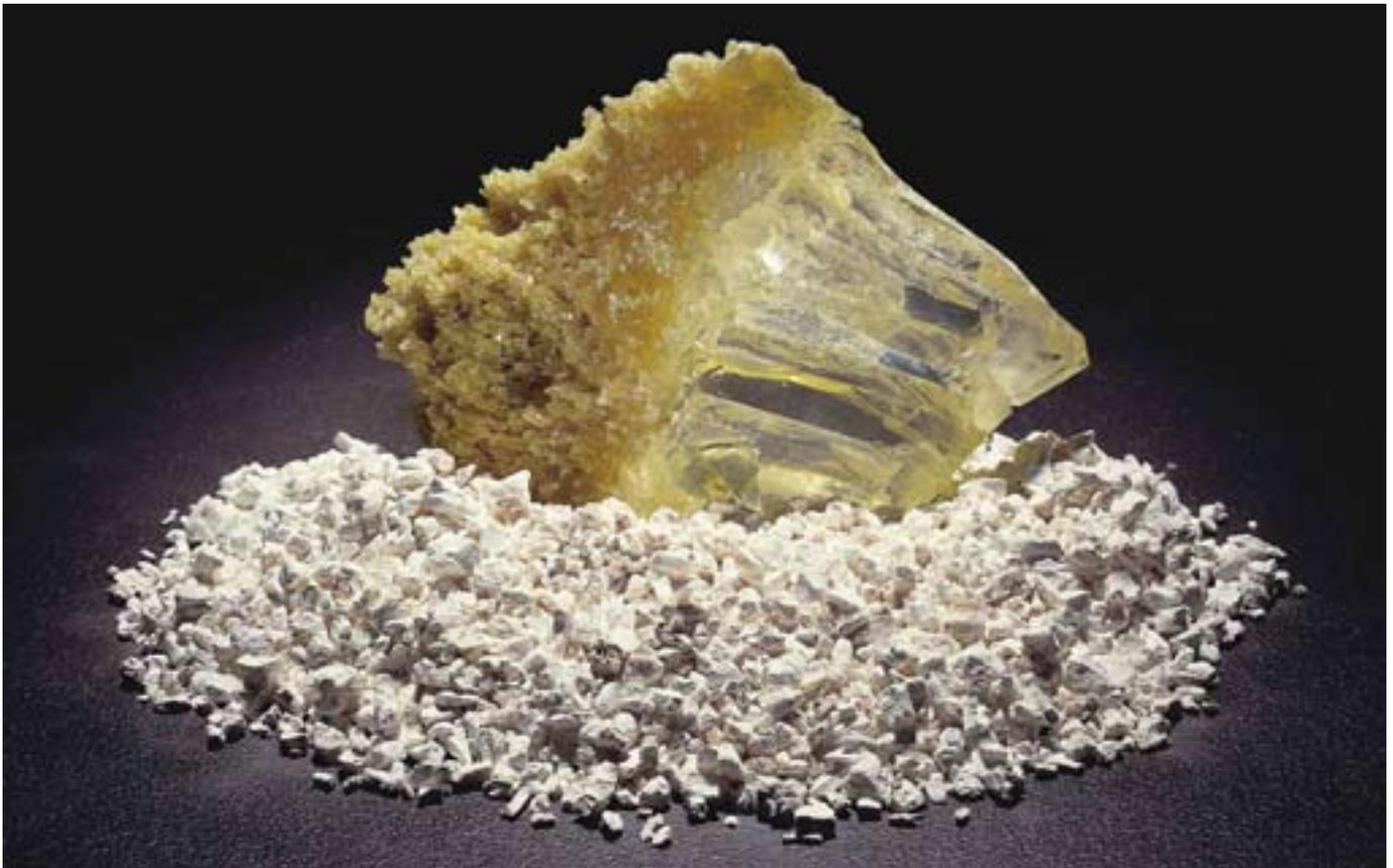
Photograph 14. Magnesite and fused magnesia. Magnesite from the Thuddungra mine is processed to caustic calcined magnesia for domestic and export markets for use in agriculture and industrial applications — mainly as a slag improver in steel making; waste water treatment; abrasives; paper manufacture; cement production; and pharmaceuticals. (Photographer D. Barnes)
