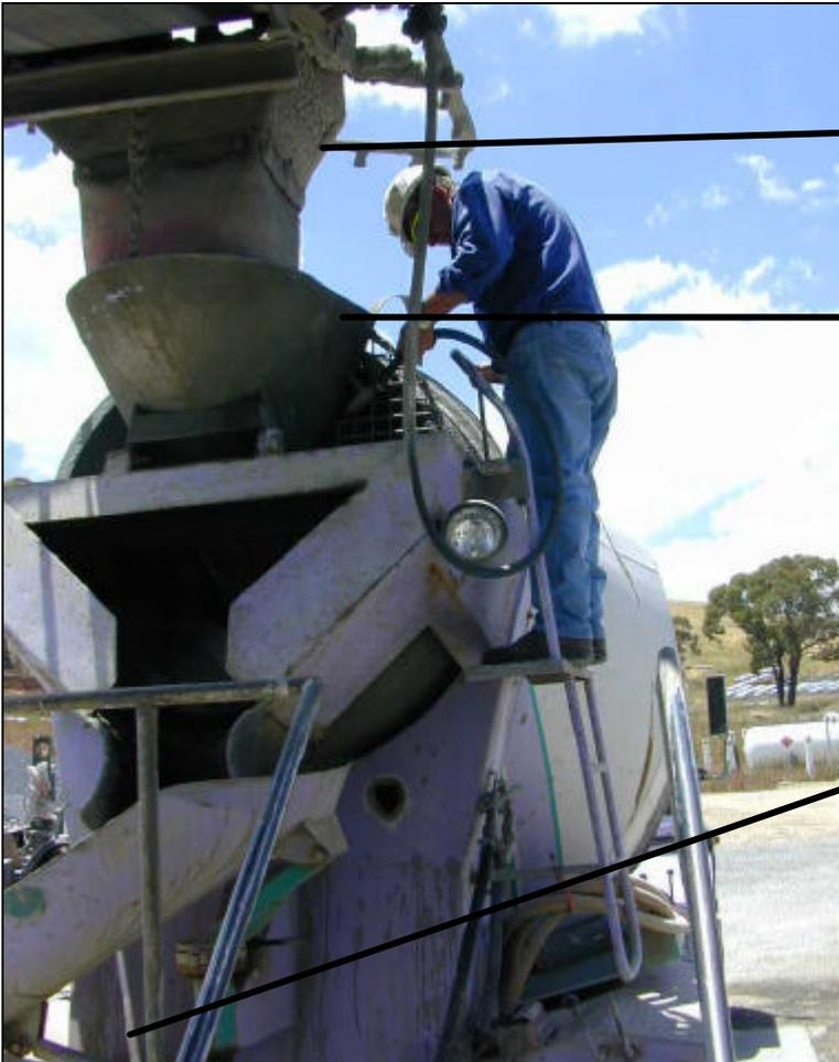
Discharge chute from batch plant conveyer above loading hopper.
