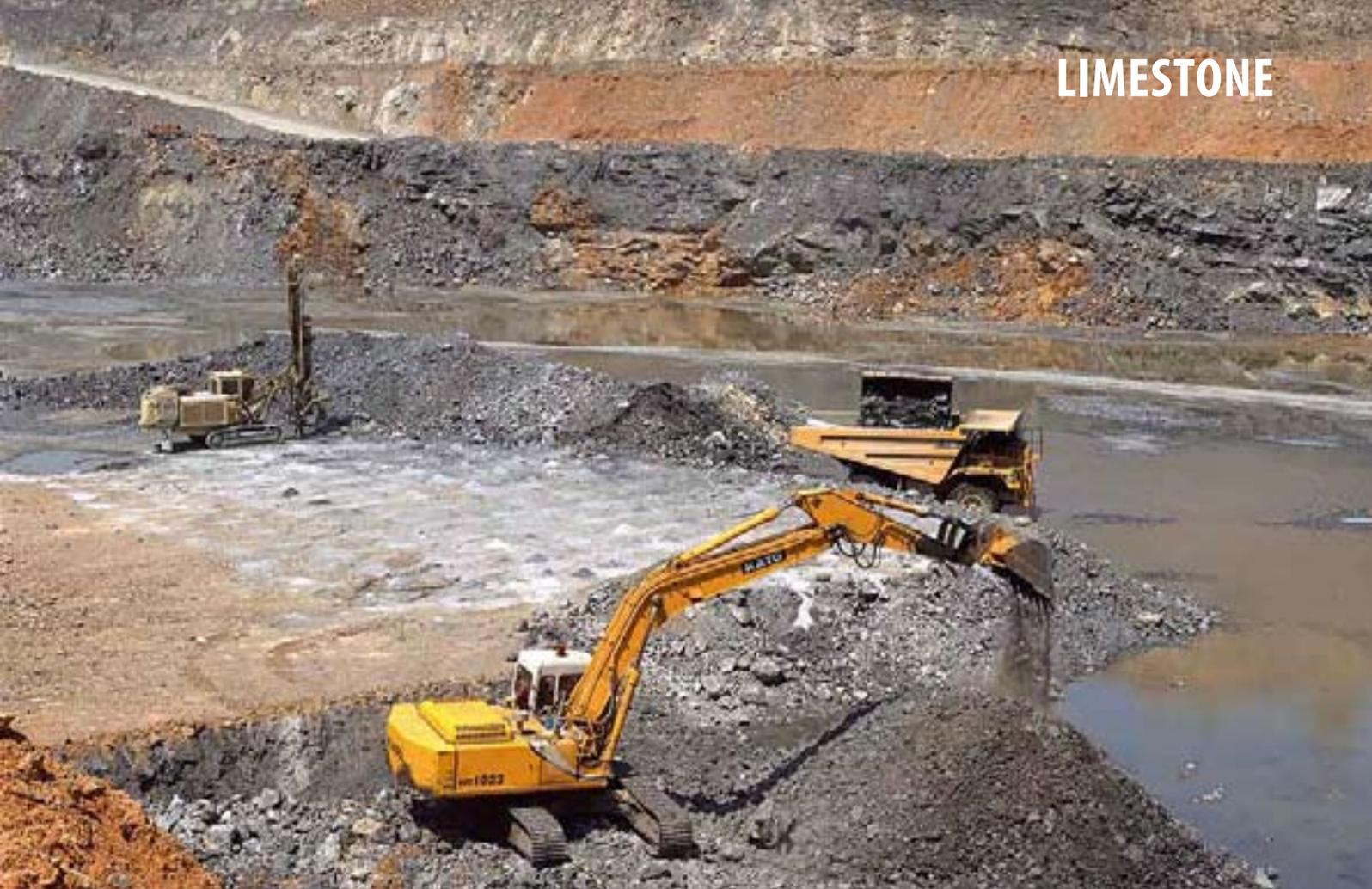
*Photograph 10. Kandos limestone quarry, Kandos. Limestone from the Kandos quarry is used in cement manufacture on-site. The ideal grade of limestone for cement manufacture is around 70–80% calcium carbonate. The Kandos plant operates two kilns, producing about 450 000 tonnes of cement each year, which is sold entirely into the New South Wales market. (Photographer D. Barnes)*
