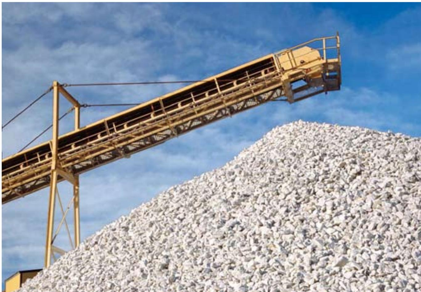
*Photograph 11. Limestone stockpile at the Omya Limited processing plant at Bathurst. Omya Southern Pty Ltd mines high-quality limestone at Cow Flat, near Bathurst. The company produces a range of ground calcium carbonate products at the on-site processing plant for use as filler materials and in chemicals. (Photographer D. Barnes)*
