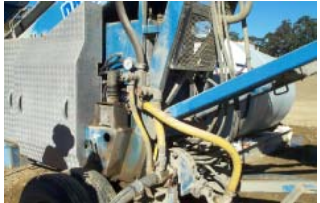
Photo above shows operator's station, water spray pump and hydraulic lines.
